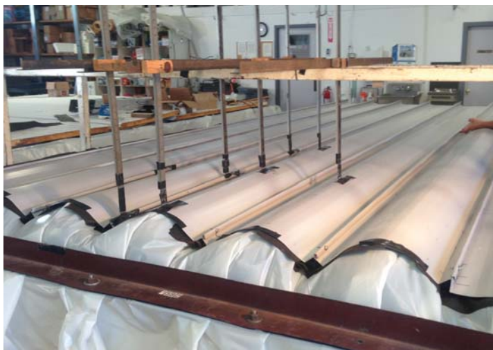
ATSM E 1592 test with pressure being applied.
