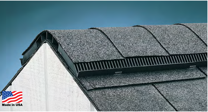
SHINGLEVENT® II 12" Filtered Shingle-Over Ridge Vent 18 sq. in. NFA per linear ft. · External wind baffle enhances airflow · Built-in ventilating end plugs · Internal weather filter helps prevent weather, insect, and dust infiltration · Limited lifetime warranty; 5-year Replacement Plus™ protection
